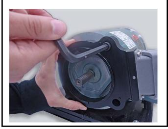
5.0 Slide Clamp wheel on to the shaft
