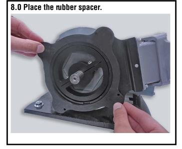
9.0 Holding the rubber spacer in place, align cover and spacer clearance holes with threaded holes on housing.
