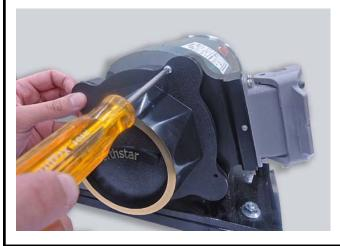
11.0 Grab mating connector, unscrew (4) mating connector screws.
