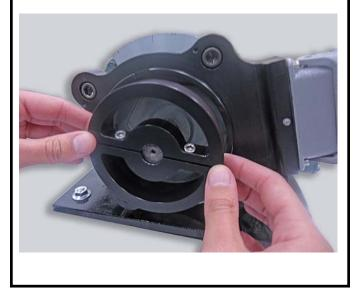
6.0 Position the wheel such that its front surface is flush with housing groove surface.
