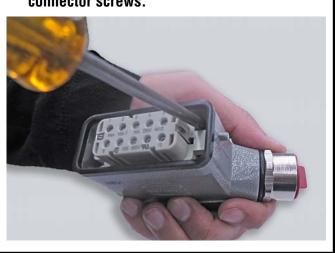
12.0 Pull the mating connector out and complete wiring per electrical connections table.
